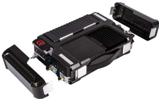
Black-side door provides access to 5915 ESR ports and Wi-Fi/cellular dongle
