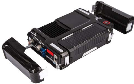
KG-250X and five additional red-side data ports accessible through red-side access door
