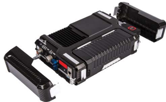
KG-250X and five additional red-side data ports accessible through red-side access door
