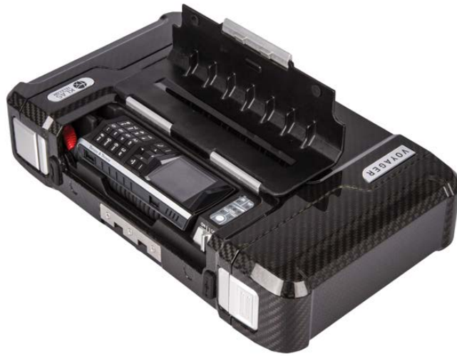
VoSIP handset and power switch accessible through side door
